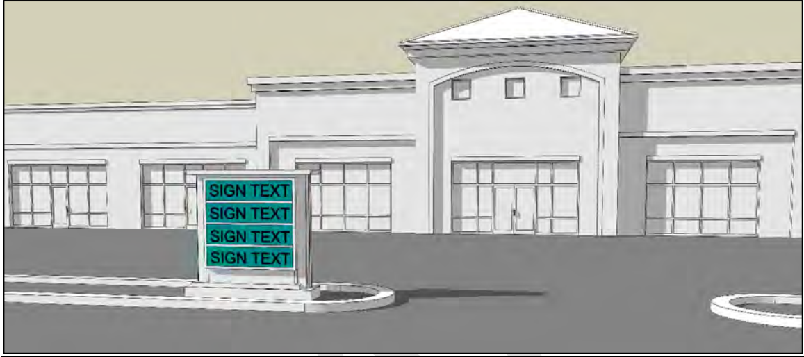
Figure 24-54: Example Monument Permanent Sign
