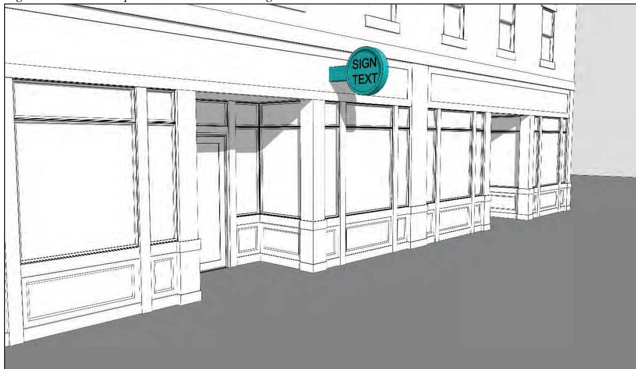
Figure 24-42: Example Blade Permanent Sign
